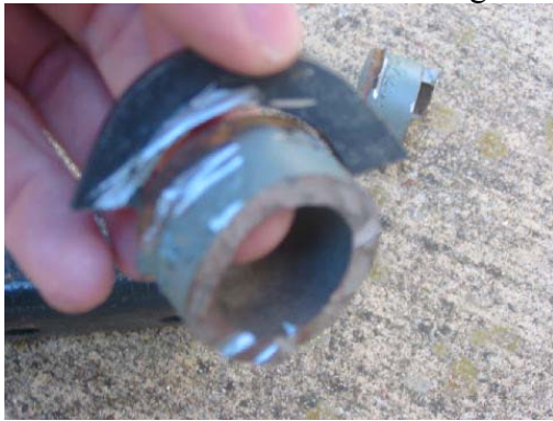
Fig 2 Areas of the cylinder where it is spot welded to the inside of the bracket. Demonstrated with what is left of the original cylinder and the new bracket.
