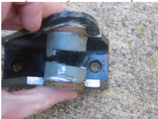
Fig 3 Old cylinder with section cut out of the middle to facilitate removal. Demonstrated with what is left of the new bracket. Do not make this cut to your new cylinder as you want to keep it intact to put in the original bracket.
