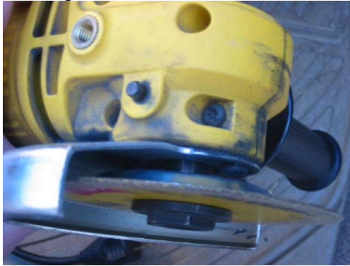
Fig 1 3 inch grinder with thin metal cutoff wheel – your primary tool
