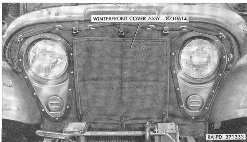
Figure 11. Winterfront cover assembly installed.
